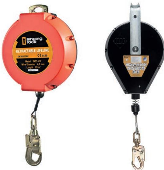
A retractable fall arrester has a similar function to the retractable safety belt in the car. Before its use it is recommended to perform a function check by slightly drawing the strap/cord and blocking it at the beginning, in the middle and at the end of its length and subsequent winding it up with control. When using a specific type of a fall arrester check whether its horizontal use (with fall factor of more than 0) is allowed.
