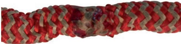
The textile equipment that has burnt or glossy surface, foto spálený textil could have been exposed to high temperatures, either by contact with a hot surface or as a result of friction with the descending device or by mutual friction of two fabrics.
