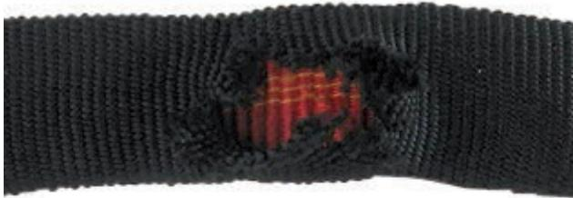
Overloading or impact loading weakens ropes and straps, and this weakening is proportional to the load to which the fabric is exposed. The ropes and straps that have been exposed to heavy loads should be retired immediately. This must be done in a way that prevents their further use.
