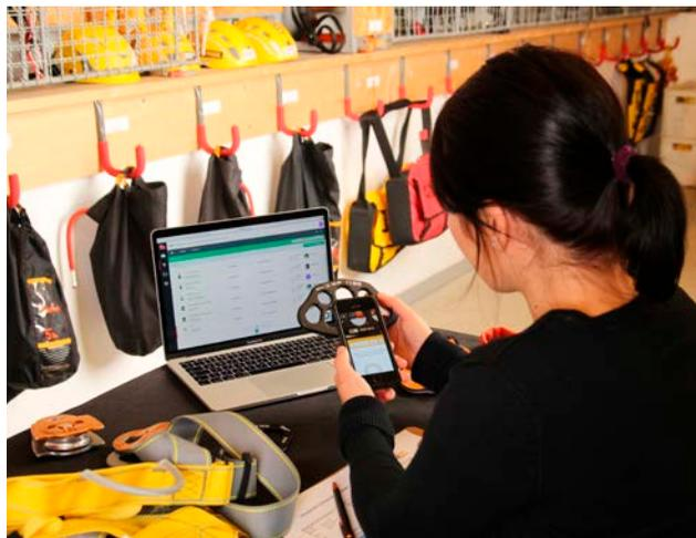
As the failure of the PPE for work at heights can cause severe injuries or death, it is essential to carry out the inspections of this equipment on regular basis. According to the EN 365 standard this inspection should be carried out by a competent person (PPE inspection technician) at least once in every 12 months. However, as this inspection does not have to be sufficient, a brief user check before every use is required.
