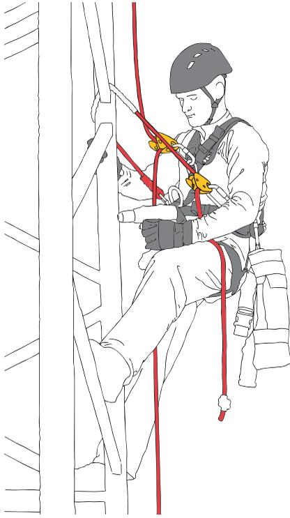
Keep in mind that the function of work positioning is not only to establish a stable working position but also to prevent any falls. Positioning side and central attachment points of the harness are used for positioning. It follows from the above stated that before starting to work a stable support must be created on the surfaces where it is missing, for example by using a work positioning harness.
