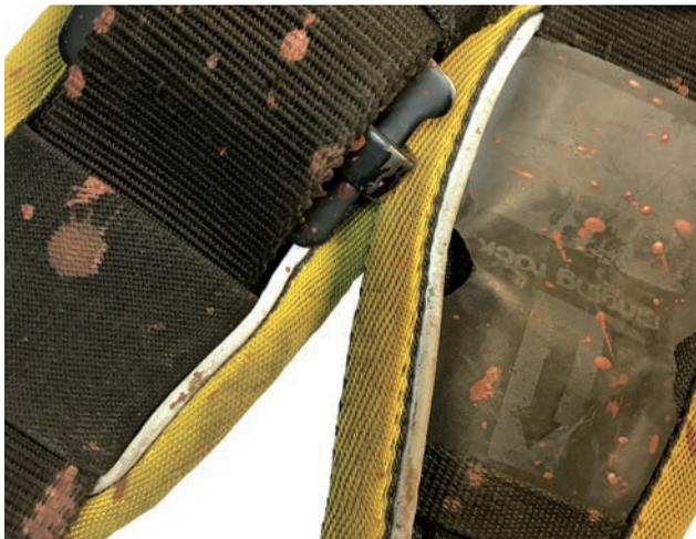
Chemical damage to textiles is often difficult to detect until the rope or strap begins to fall apart and therefore can be overlooked during the inspection. It may be indicated by white powder residue on the surface of the fabric or a significant change in texture. foto chemické poškození
